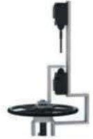
Limit Switch Arrangement
